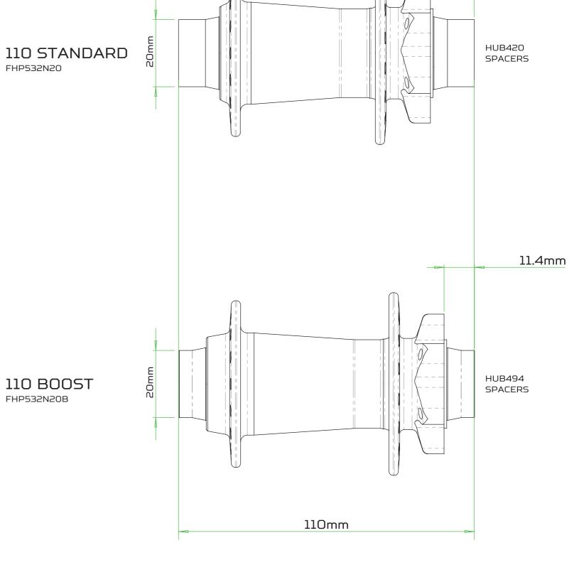
110 BOOST 11.4mm Disc offset (Distance from dropout to flange) 16.4mm
