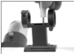
Fig. 10: Attach the viewfinder bracket to the optical tube.
