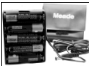
Fig. 12: Insert 10 AA batteries into battery pack.
