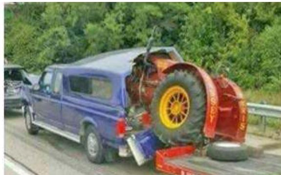
As an added note, when I tie down a tractor, I always use my strongest chains to keep the tractor from going forward on the trailer. There should be one on each side of the tractor to the trailer side.
