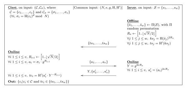
Figure 2: APSI Protocol from [17] (simplified for semi-honest security). The protocol is run on common input of RSA modulus N=pq (with p and q safe primes), public exponent e, a random element g in  $\mathbb{Z}_N^*$  and two hash functions, H and H', modeled as random oracles. All computation is mod N.
