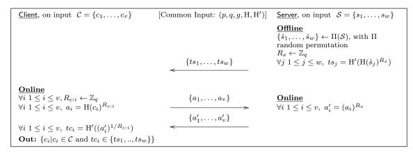
Figure 3: PSI Protocol from [44] (simplified for semi-honest security). It runs on common input of two primes p and q (s.t. q|p-1), a generator g of a subgroup of size q and two hash functions, H and H', modeled as random oracles. All computation is mod p.
