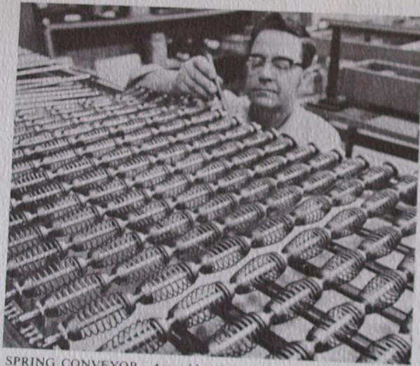
SPRING CONVEYOR - Assembly of the conveyor using Egomatic stainless steel spring rollers.
